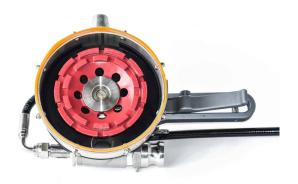
DOUBLE ROW 125MM DIAMOND CUP WHEEL (FOR GRINDING CONCRETE SURFACES).
